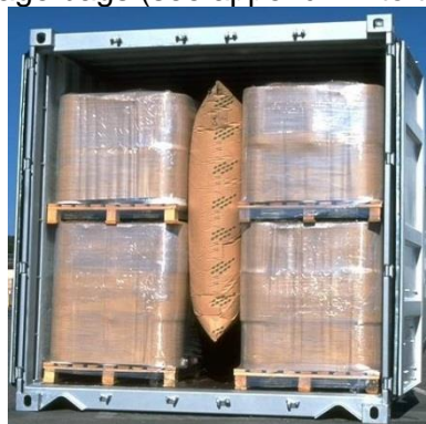
Figure 7.9 Gap filled with a central dunnage bag
