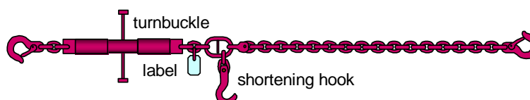
Figure 7.18 Standard chain lashing with shortening hook
